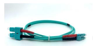
The duplex fiber patch cord is OM3 with 3 mm jacket. It is LSZH rated and its terminated with LC fiber optic connector on one end and SC fiber optic connector on other end.
